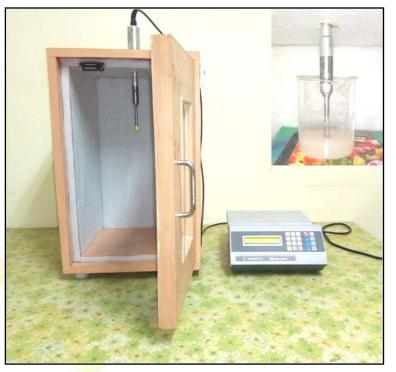
HAP/PCS and mineral substituted HAP/ PSSG etc.) and Sonicators have become the nanotechnology standard for Dispersing, Deagglomerating, Particle size reduction, Particle
